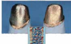
Captek G after firing Captek G melts over Captek P capillaries forming the internal supporting skeleton.
